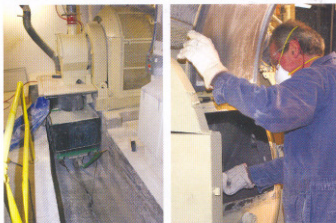
The batch is rapidly discharged from the mixer into a cart that transports it to the furnace.
