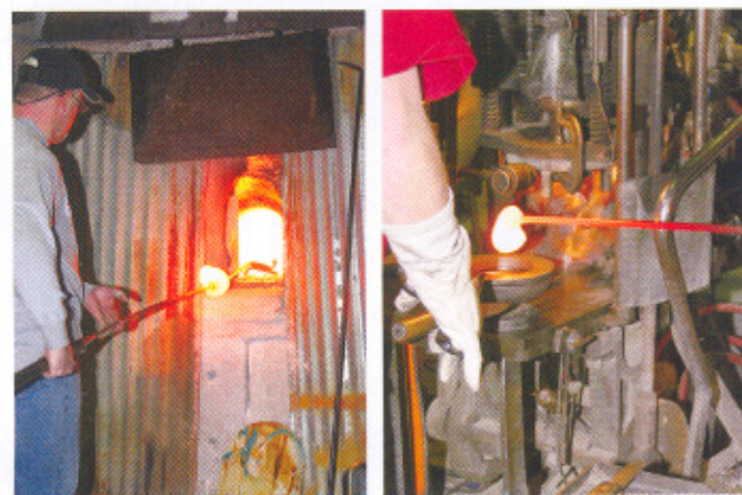
The gatherer uses a punty, which is continually turned, to accumulate molten glass from the pot, and transfer it to a mould.
