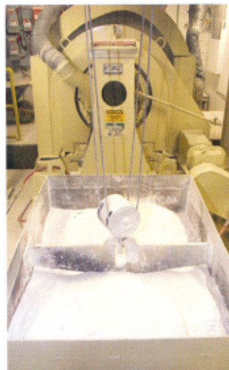
The flange of a discharge valve at the hopper's outlet is positioned atop the inlet of the mixer using an overhead hoist and trolley, due to ceiling height restrictions.
